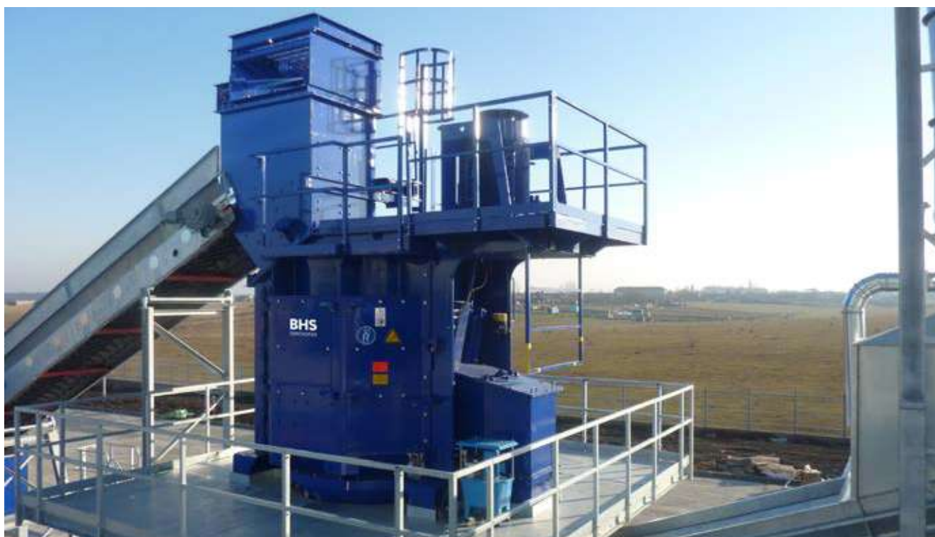
The E-Scrap plant in Romania is centered on a Rotorshredder of type RS 2018.
