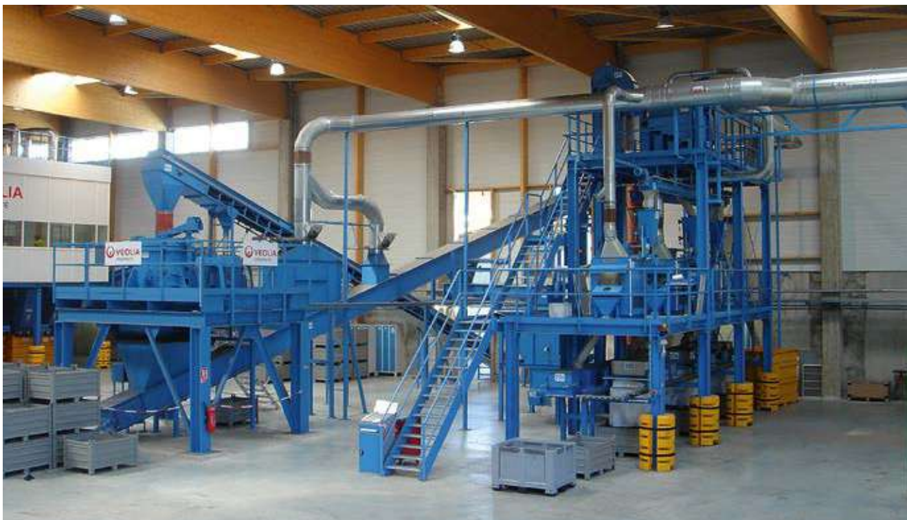
The second major component of an E-Scrap recycling plant can be a BHS rotor impact mill of type RPMV 1113 for fully mechanized treatment of the 0-20 mm fine fraction in the second stage.
