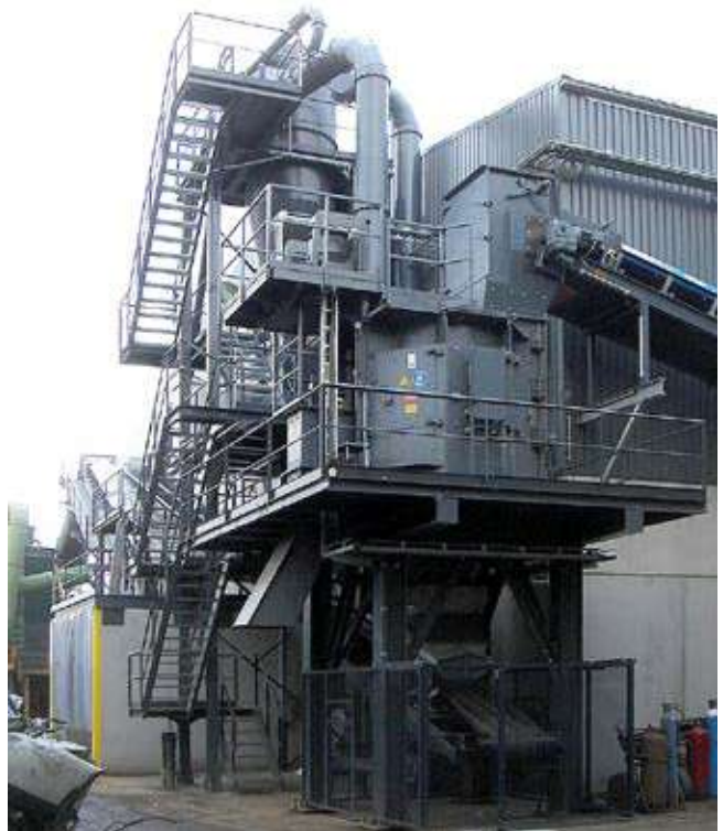
This Rotorshredder of type RS 2018 is used in France for the metal recycling of shredder fractions.
