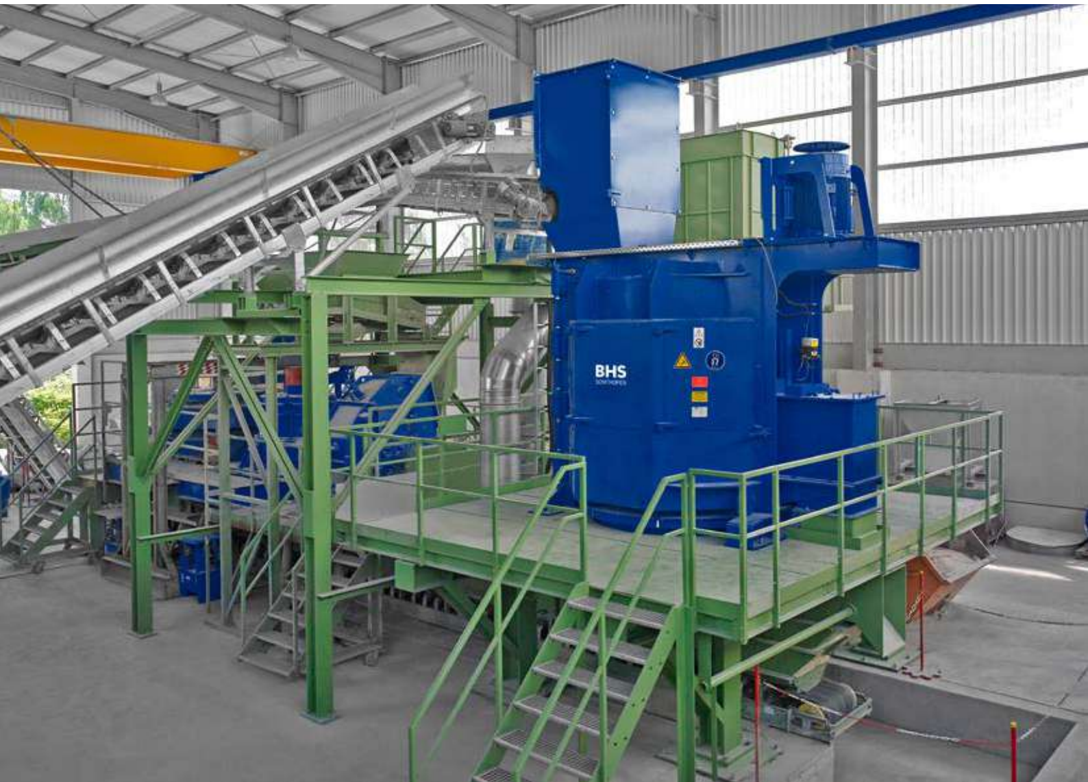
Rotorshredder of type RS 2018 for tests at the BHS technical center at Sonthofen.
