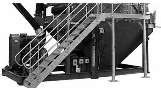
Galvanized walkway, steps and handrails included standard with all machines
