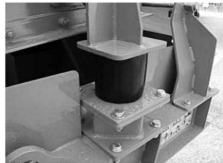
High efficiency rubber screen mount for minimal vibration transfer
