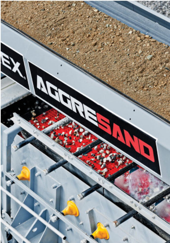
Aggregate Screen Fitted with Isolated Spraybars
