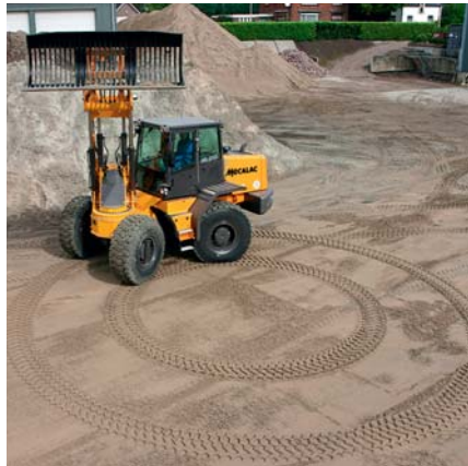
4.90 m turning radius measured over rear end
